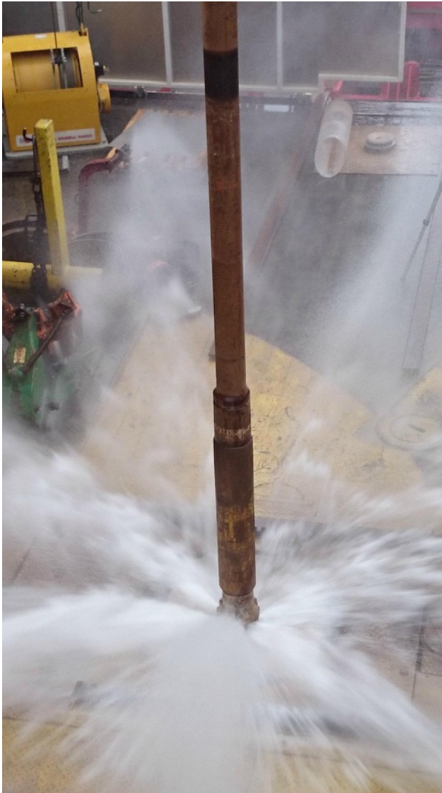
Figure 5. The Afterburner aims to replace cuttings cleaning by jet impact. This picture shows the jet impact from a rate of 1600 lpm.
