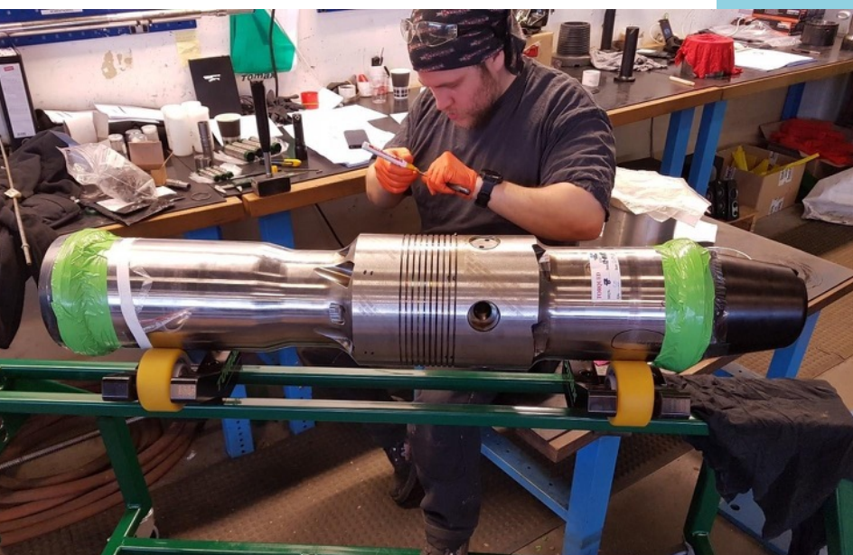
Figure 4. 2018 version Afterburner with wire-feed for integration in commercial RSS system.
