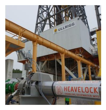
Figure 5 Pilot-scale HeaveLock<sup>™</sup> prototype, ready to be tested at IRIS Ullrigg in Stavanger
