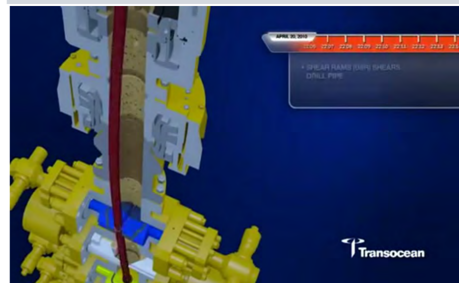
Deepwater Horizon BOP - reconstruction of blowout (courtesy Transocean)
