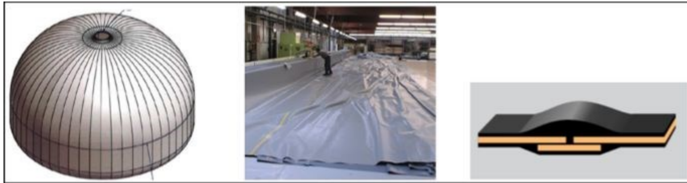
Figure 5 - Flexible bag design, production of bag, principle for vulcanizing sheets
